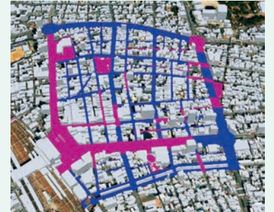
Visualized the relationship between pedestrian flow and heat stress by overlaying the results of thermal environment analyses with human occupancy data.
